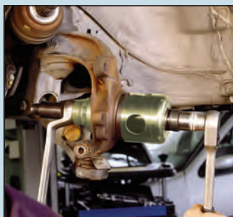
Higher axial forces in spite of lower application of force (due to high capacity threaded spindle with special trapezoidal fine thread in conjunction with the axial cylinder roller bearing)
