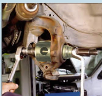
O-ring-clamping developed by HAZET retains the thrust washer on the centering bushing when installing and removing the wheel bearing.
