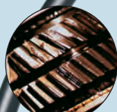
Gear damages and wear marks
