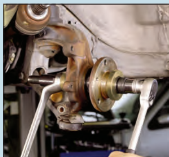
Optimal centering when inserting the wheel hub into the new wheel bearing
